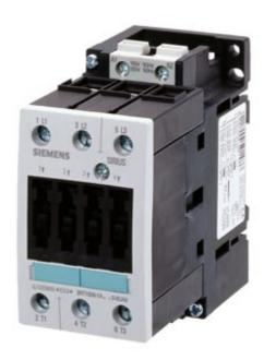
CONTACTOR, AC-3 15 KW/400 V, AC 24 V, 50 HZ, 3-POLE, SIZE S2, SCREW CONNECTION
