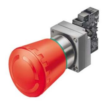
22MM METAL ROUND COMPLETE UNIT COMBINATION: EMERGEN.-STOP MUSHR.PUSHB. 40MM LATCH.W. ROT. -TO-UNLATCH MECH. WITH YELLOW BACKING PLATE SCREW TERMINAL, 1NO+1NC WITH HOLDER RED INSCRIPTION: EMERGENCY STOP
